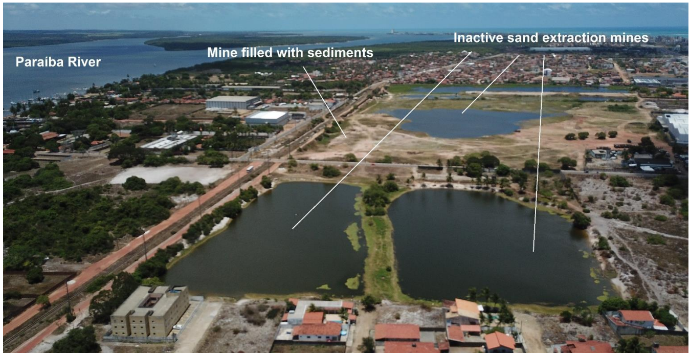
Figure 6. Inactive sand extraction mines in Cabedelo. The mined areas are full of water due to having reached the water table, which in this area is extremely shallow. Photo: Authors (2020) (Use of drone). Photo taken from south (foreground) to north (background).
