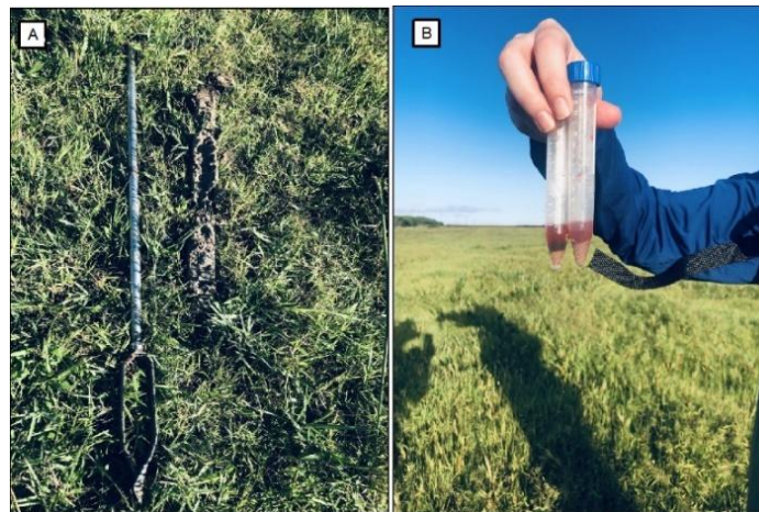
Figure 3. Assessment of hydromorphic soil: A) sampling with an auger; B) application of a,a'-dipyridyl, a pedoenvironmental indicator for hydromorphic soils. Photo: by the authors.
