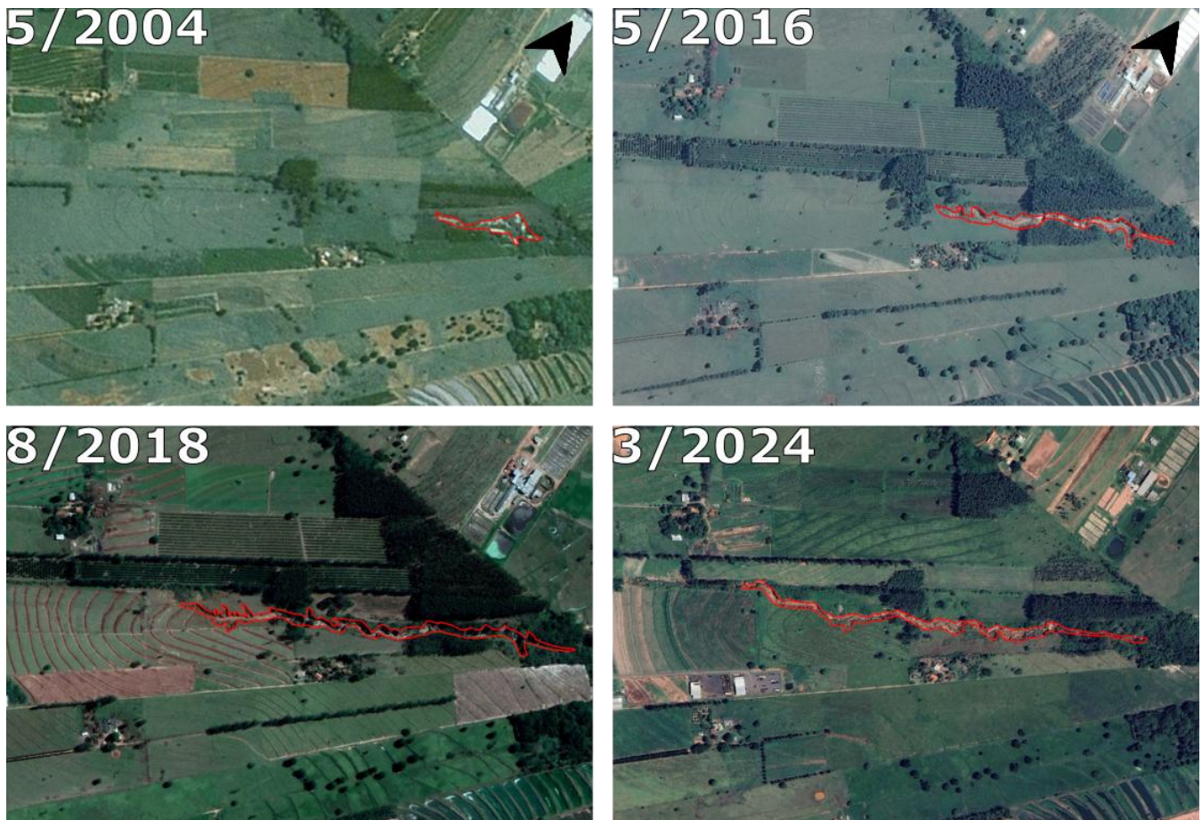
Figure 8. Evolution of Gully in the district of Sumaré, Paraná (latitude: 23° 4'35.79"S; longitude: 52°23'37.74"O). In red perimeter of the gully over the years. Source: Google Earth pro
